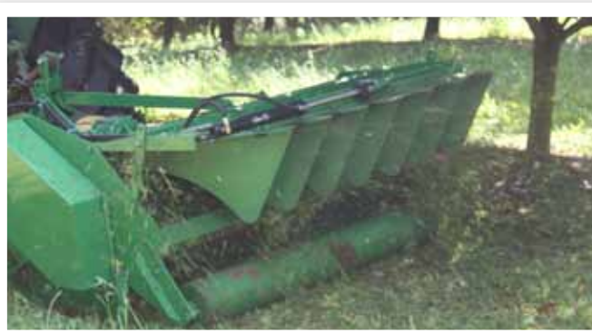
Under tree mulcher showing deflecting veins
